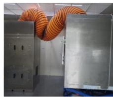
1 INDOOR AC TESTING CHAMBER WITH NOZZLE SIZE ADJUSTMENT
